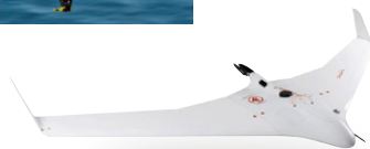
BRAMOR ppX for surveying
