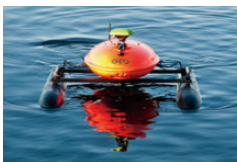
Autonomous, remotely operated USV (SONOBOT)
